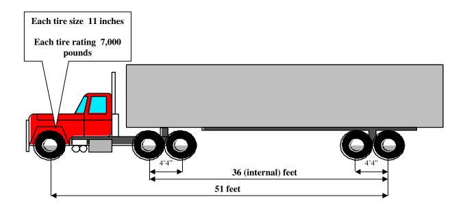
Allowable steering weight by size = 13,200 # weight by rating = 14,000 #
